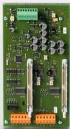
Customer-specific floor plan displays are possible thanks to the C-NET-powered mimic display driver FT2001-A1.
